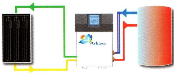
Figure 2: Basic layout of the solar-assisted heat pump, with the solar thermal panels on the left and the smart box in the centre
